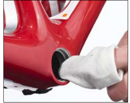
Figure 39. Cleaning bonding surfaces with an alcohol wipe
